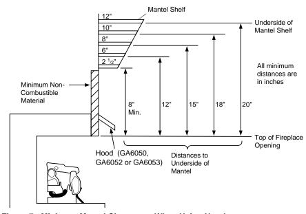
Figure 7 - Minimum Mantel Clearances When Using Hood
